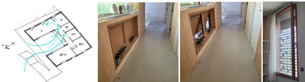
Figure 7. Left: plan view of Baitykool Living Lab with night ventilation strategy, Right: Image of Patio Ventilator with closed, open position & window in open position.
