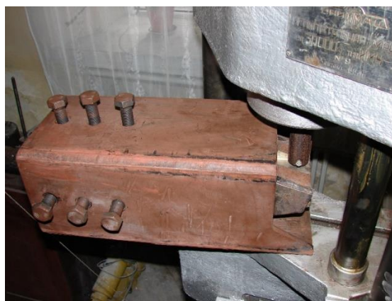
Figure. 13: Dynamometric tooth calibration in laboratory
