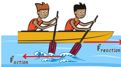
Figure 2. Illustration the Action and Reaction Forces on a Boat Being Rowed
