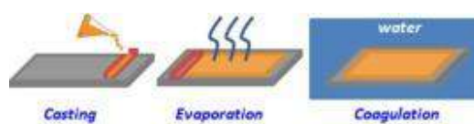
Figure 7: Schema of Membrane Fabrication Method
