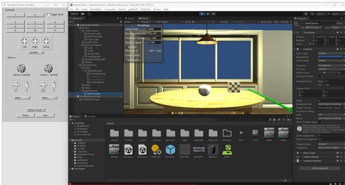
Figure 2. Completed scene showcasing the use of trackd to simulate getReal3D VR controls within the Unity Editor
