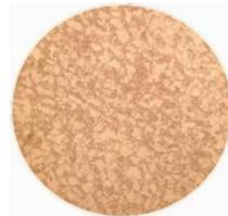
Figure 9. Micrograph for Carbon Steel which was Heat Treatment with Normalizing X: 160
