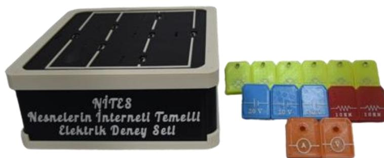
Figure 1. IoTES (Internet of Things-Based Electricity Experiment Set)
