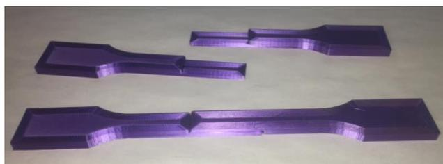
**Figure 5:** 3D printed single lap shear joints
