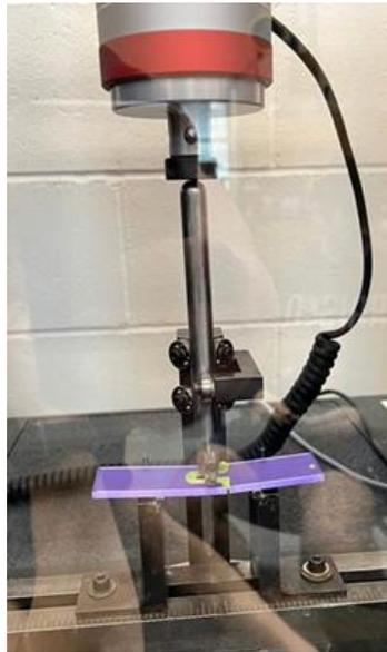
**Figure 8:** 3-pt flexural testing of weld joint
