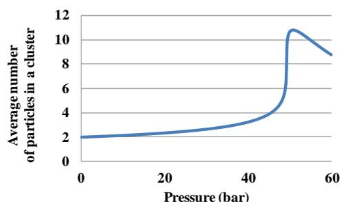
Figure 3. The basic particles average number in an Argon cluster at a supercritical temperature,  $T = 151$  K.
