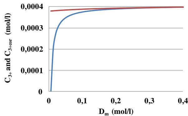
Figure 3. Large errors in the initial  $C_{3+}$  values (blue line), corrected by the reverse analytical extension method: corrected values  $C_{3+cor}$  (red line).
