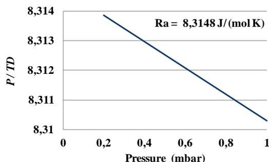
Figure 11. Estimation of the apparent gas constant  $R_a$  for Helium data from the NIST Webbook (NIST 2021).
