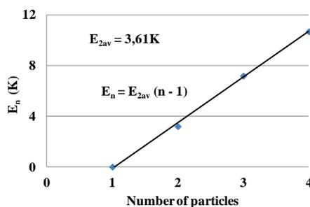
Figure 8. The linear Helium small clusters' bond energy  $E_n$  dependence on the number  $n$  of particles in a cluster.
