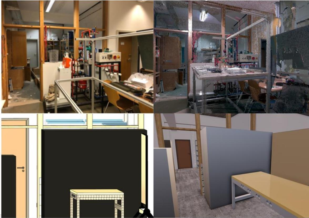
Figure 3. Example of one of the rooms and the results: Photography of the actual state in the beginning (top left), recorded point cloud data (top right), three-dimensional model for planning purpose in Revit (bottom left) and three-dimensional virtual reality model in the target state (bottom right), own representations.
