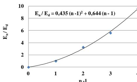
Figure 9. The quasi parabolic bond energy  $E_n$  dependence on the number  $n$  of particles in an Argon cluster.
