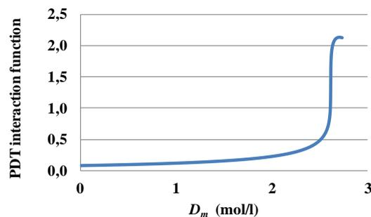
Figure 4. The Pressure-Density-Temperature (PDT) interaction function  $C_{2+} = (D - D_p)/D_m^2$ .
