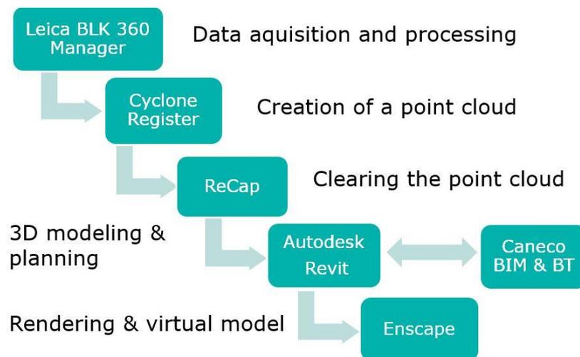
Figure 2. Overview of the workflow, the software used and the work steps, own representation
