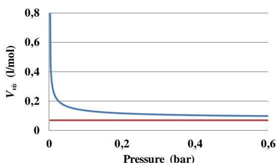
Figure 10. The characteristic viscosity volume  $V_{vis}$  dependence on pressure for Xenon at 180 K (blue line) and Krypton at 150 K (red line).
