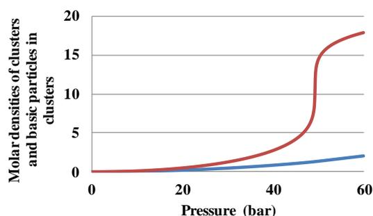
Figure 2. The total density of basic particles contained in clusters ( $D - D_m$ ) (red line) and the molar density of clusters ( $D_p - D_m$ ) (blue line) in Argon at a supercritical temperature,  $T = 151$  K.
