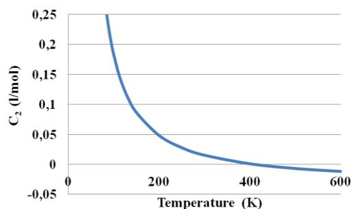
Figure 5. The temperature dependence of the apparent equilibrium constant for dimers in Argon.
