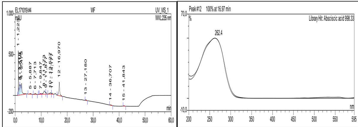
**Figure 3A & 3B. HPLC Chromatogram and UV Spectrum of Peak 12 respectively, suggesting Abscisic acid at 235 wavelength. Key: WF= water fraction**
