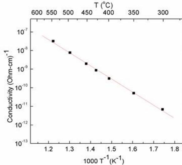
Figure 3. Conductivity of heteroepitaxial diamond vs.  $T^{-1}$ . An activation energy of  $1.40 \pm 0.03$  eV is found for heteroepitaxial diamond from the linear fit (solid line).
