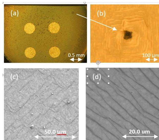
Figure 1. Optical microscope image of (a) the free-standing sample at 5X with average diameter of 3.5 mm and an array of four 0.5 mm diameter Ti/Au electrodes, and (b) spiral type defect with average size of  $\sim 50\text{-}100\ \mu\text{m}$  at 20X; SEM images of diamond surface (c) near the center showing inclusions and screw dislocations, and (d) away from the center with fewer defects showing macrosteps parallel to [110] with an average size of 5  $\mu\text{m}$ .
