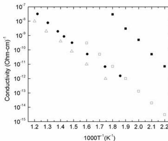
Figure 4. Comparison of temperature-dependent conductivities of heteroepitaxial ●, natural Type IIa Δ [1], Type IIa □ and Type Ib diamond ■ [10]. VZ and BW plots are reconstructed from VZ report Figure 4 [1] and BW report Figure 1 [10], respectively
