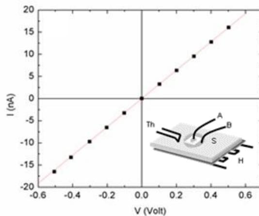
Figure 2. I-V characteristics of heteroepitaxial diamond with Ohmic Ti/Au and Ir contacts at 545 °C, and Inset: sample holder schematic; Sapphire 10 mm square; white square, the diamond sample; A, Au-wire contacting top electrode; B, Au-wire contacting Au-pad; Th, Thermocouple; S, Sapphire; H, Heater.
