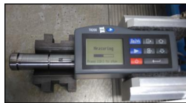
Figure 3. Rugosimeter measuring the Roughness of a Specimen
