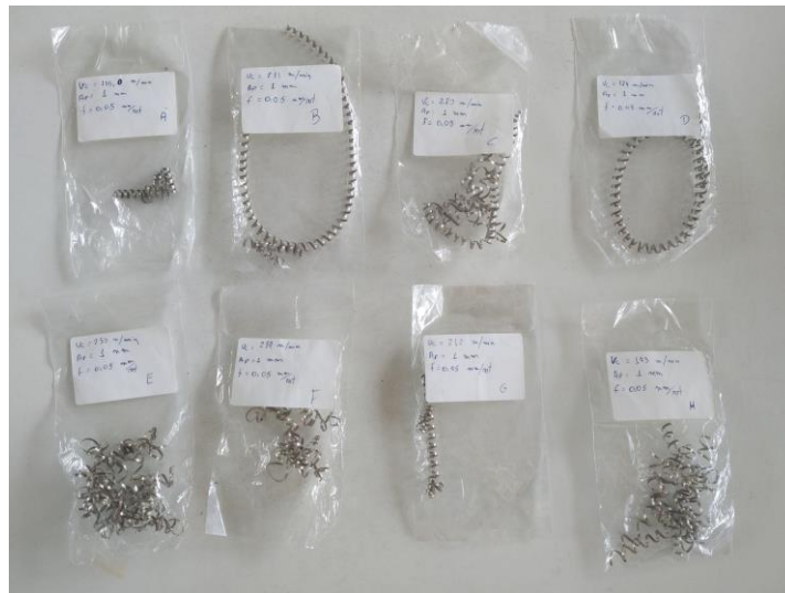
Figure 5. Sample of Chips collected after Machining Parts
