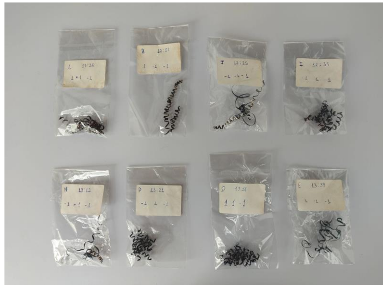
Figure 5. Collected Chips after Machining Parts
