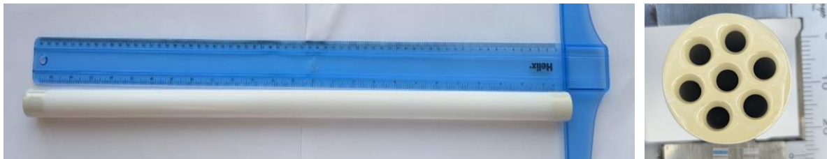
Figure 7. Ceramic Support: Total Length (left) and Internal Channels (right)
