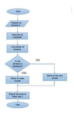
In this algorithm K data elements are selected as initial centers and Euclidean distance formula is used to calculate the distance between the selected centroid and other data elements and then same procedure is followed iteratively.
