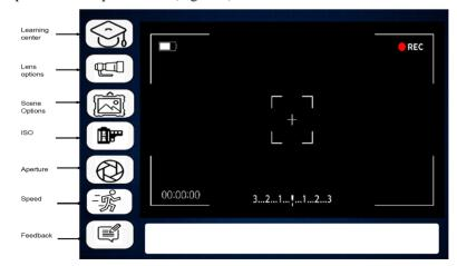
Figure 4. Interface for our proposed VR based Photography Training Simulator
