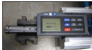
Figure 3. Rugosimeter measuring the Roughness of a Specimen
