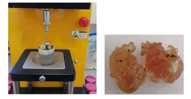
Figure 1. a) Cement Mortar Sample on Table TA-BT-KIT about to be tested. b) AG Tears
