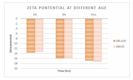
Figure 2. Zeta Potential of AG dissolved in Water and Lime Water
