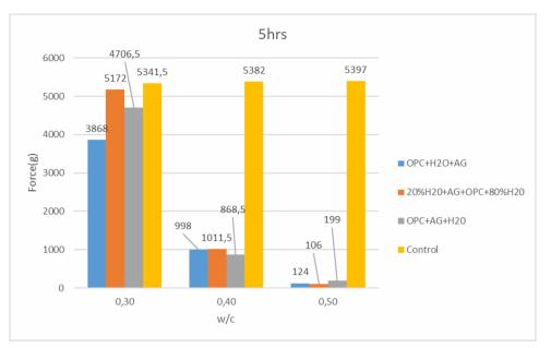
Figure 6. Force of Indent versus w/c at 5 hrs of Age
