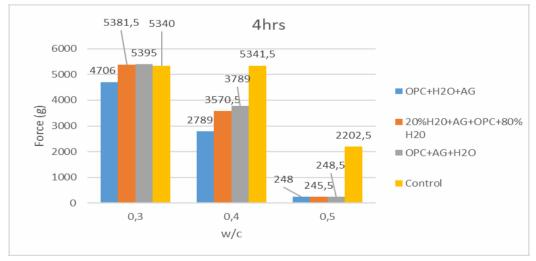
Figure 5. Force of Indent versus w/c at 4 hrs of Age
