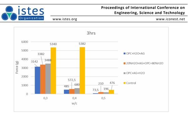
Figure 4. Force of Indent versus w/c at 3hrs of Age
